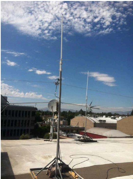
Comet GP1, Alpha Delta DX LB & Comet CHV5x in foreground and Comet GP3 & Radiowavz OCF 80 in background
