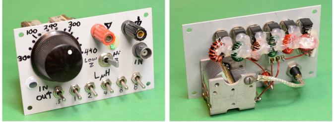
Front and back of the Tuner. This version has an extra 8µH inductor, that has never been needed, and is used with an external SWR metering circuit. The variable capacitor is a 30pF to 440pF unit.
