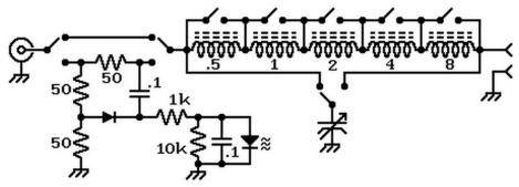
The Variable Inductance is obtained by switching in or out fixed inductors with values in a binary sequence, giving half microHenry accuracy to a maximum of 15.5 microHenrys. The switches are miniature toggle switches rated at 120V and 5A.
