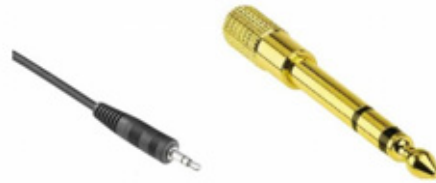
headset audio cable (left) and dollar-store adapter (right)
