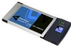
The computer industry embraced the concept with open arms and has continually refined the technology to the point that sub-\$100 equipment is now available capable of sending 11 million bits/sec in the 2.4 GHz band.
