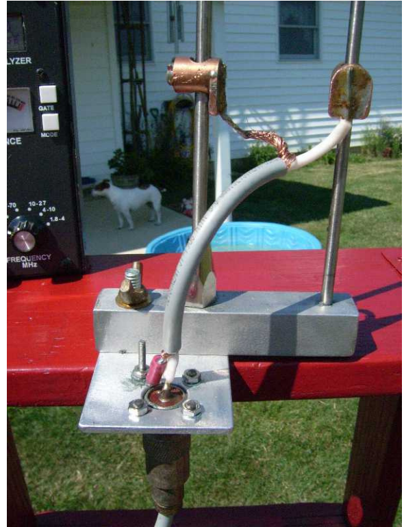
Rear view of coax taps & SO-239 connections
