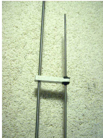
Speed nuts trap the spacer.
