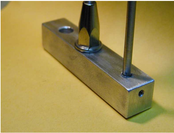
Mobile J base block is an aluminum \frac{3}{4} " SQ x 4" bar.
