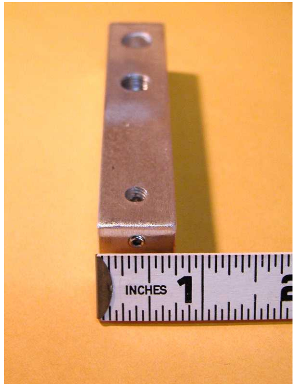
Mobile J base block is an aluminum \frac{3}{4} " SQ x 4" bar.
