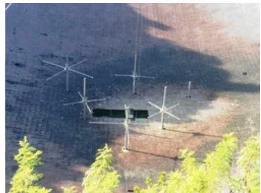
The triangular 5.1 MHz and 8.175 MHz dipole array in the dish. [Courtesy of Jim Breakall, WA3FET]
