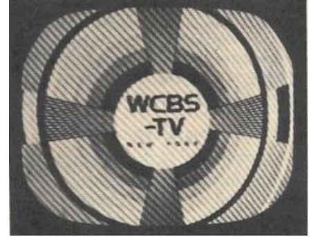
An example of TVI on VHF channel 2. [ The Radio Amateur's Handbook - 1972]
