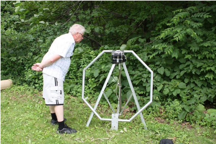
Now that looks interesting. John Visser, VE3FDV examining a magnetic loop antenna before it got set up. (VE3IDT)
