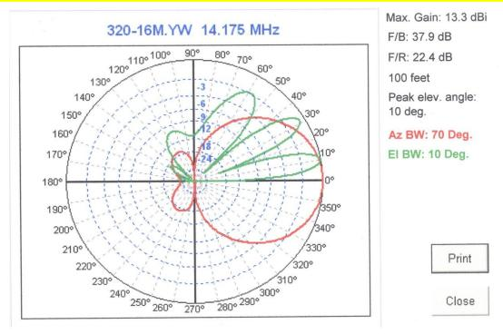
I took the relative gain in  $5^{\circ}$  steps off of the plot, added it to the max gain of 13.3 dBi and subtracted the 2.15 dB correction factor for dBi to dBd to generate the 100 ft. Yagi column in Table 3 below. Similar runs on YW at 33 and 66 ft. height and Dipoles on EZNEC at 33 ft. fill out Table 3.
