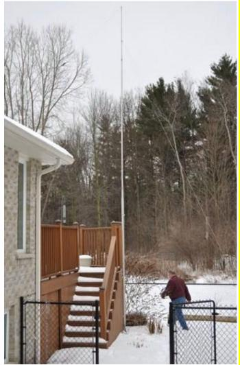
Antenna. Guy wires come down to fence at right
