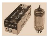
The valve line up was as follows: 3S4 RX RF amp, TX RF Power amp; 1R5 RC Mixer/Osc, TX Crystal Osc; 1T4 RX IF amp, TX not used; 1S5 RX Detector/AVC/AF amp, TX Mic preamp; 3S4 RX AF output stage, TX Choke modulator. In order to preserve 1.5 volt 'A' battery life only one half of the 3S4 filaments were used during receive and the
