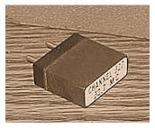
As an aside, Galvin also coordinated 30 other manufacturers, implementing quantity production techniques, which resulted in the eventual delivery of 35 million quartz crystal units (shown to the left) during WW II.
