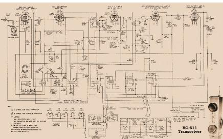
The receiver was a single conversion superhet using a 455 KHz IF stage with a RF amplifier. This configuration opposed the trend of the day where similar infantry equipment using regenerative receivers was the norm. Not only did the SCR-536 use а superhetrodyne design but it also had the high receiver performance (for its time) which a RF amplifier stage could provide. Galvin achieved all this in such a small package by building one of the first true
